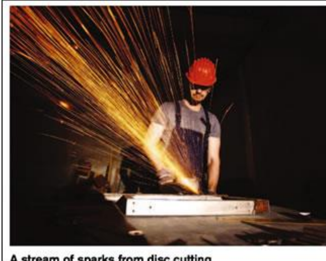
A stream of sparks from disc cutting
